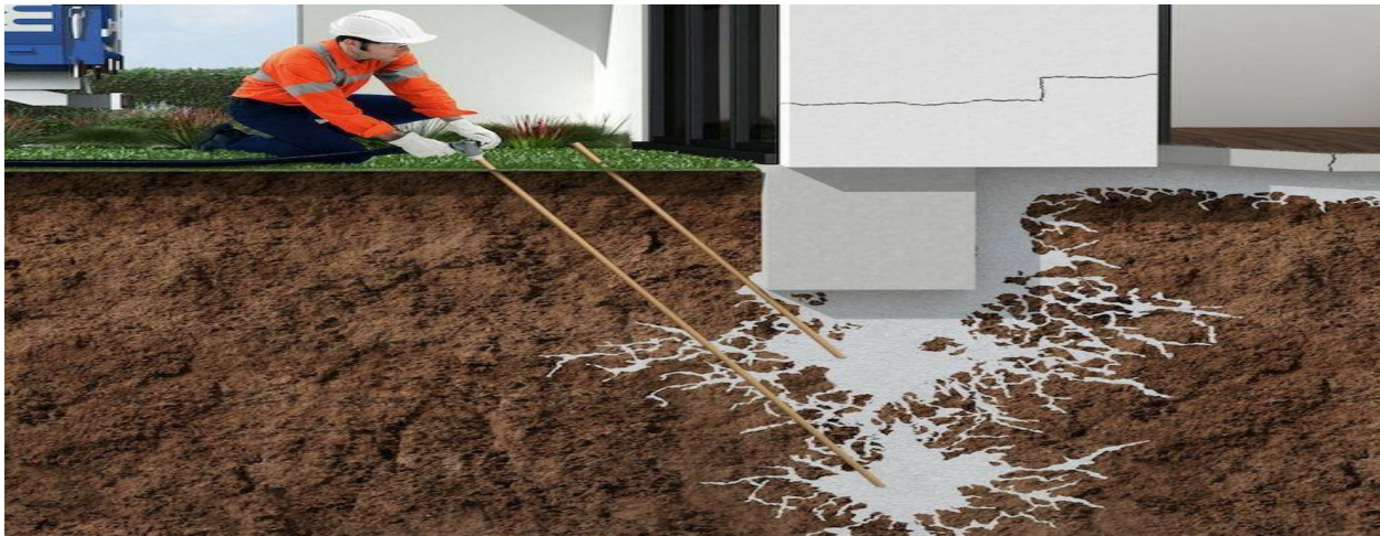
Fig.8: chemical Underpinning Method
